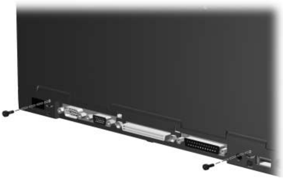
Figure 5-22. Removing the Switch Cover Screws
