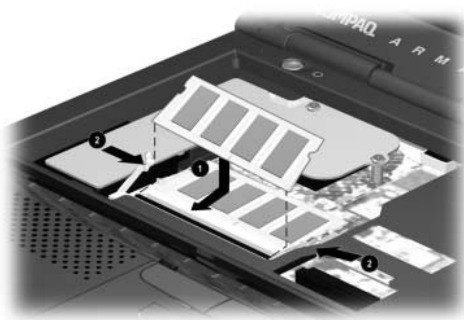
Figure 5-21. Installing a Memory Expansion Board
