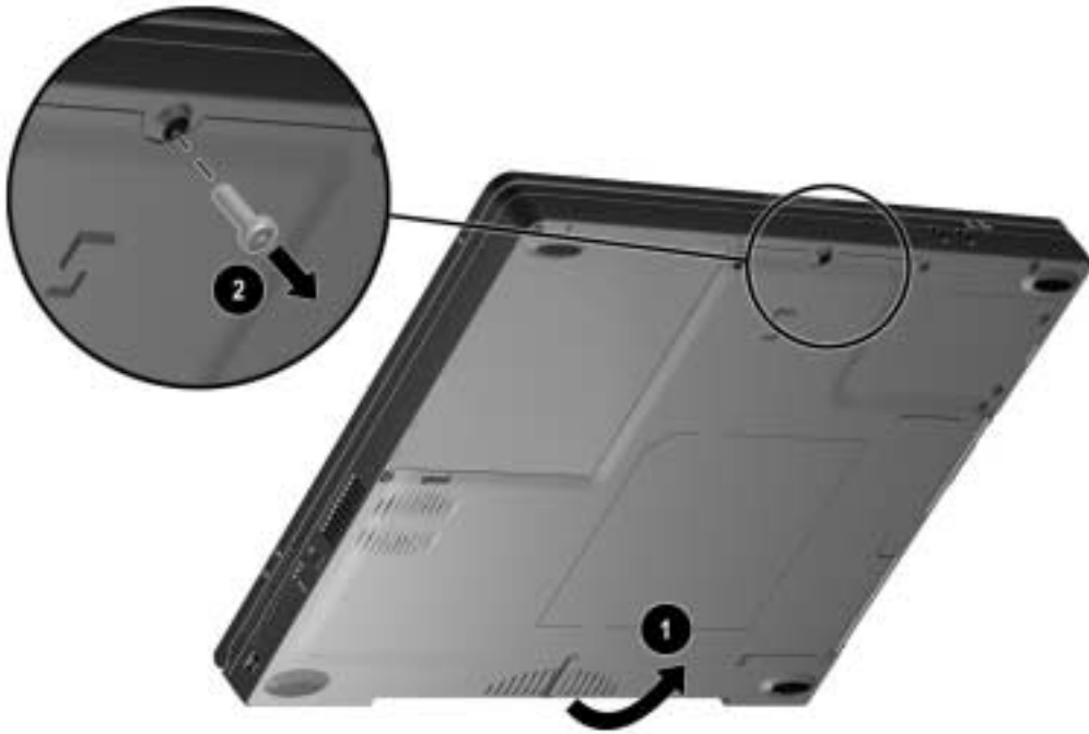
Figure 5-7. Removing the Hard Drive Screw
