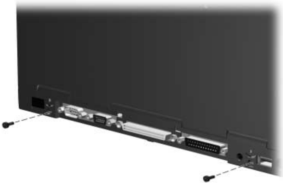
Figure 5-25. Removing the Display Assembly Screws
