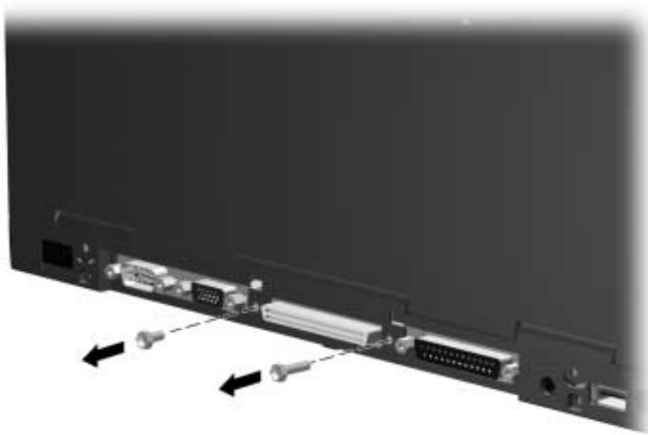
Figure 5-34. Removing the Bushing Guides
