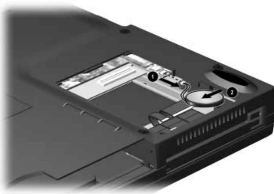
Figure 5-17. Disconnecting the RTC Battery Cable
