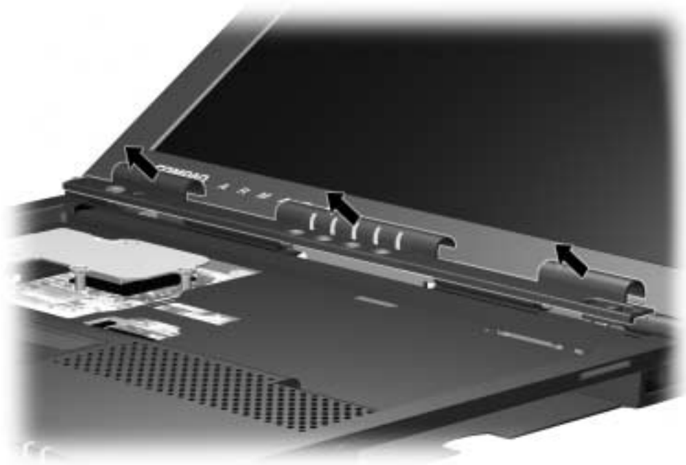
Figure 5-23. Removing the Switch Cover
