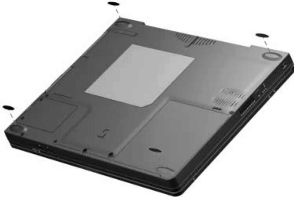
Figure 5-4. Installing the Computer Feet
