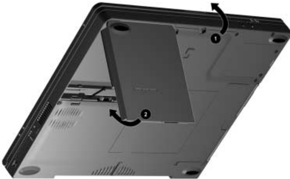
Figure 5-6. Inserting a Battery Pack
