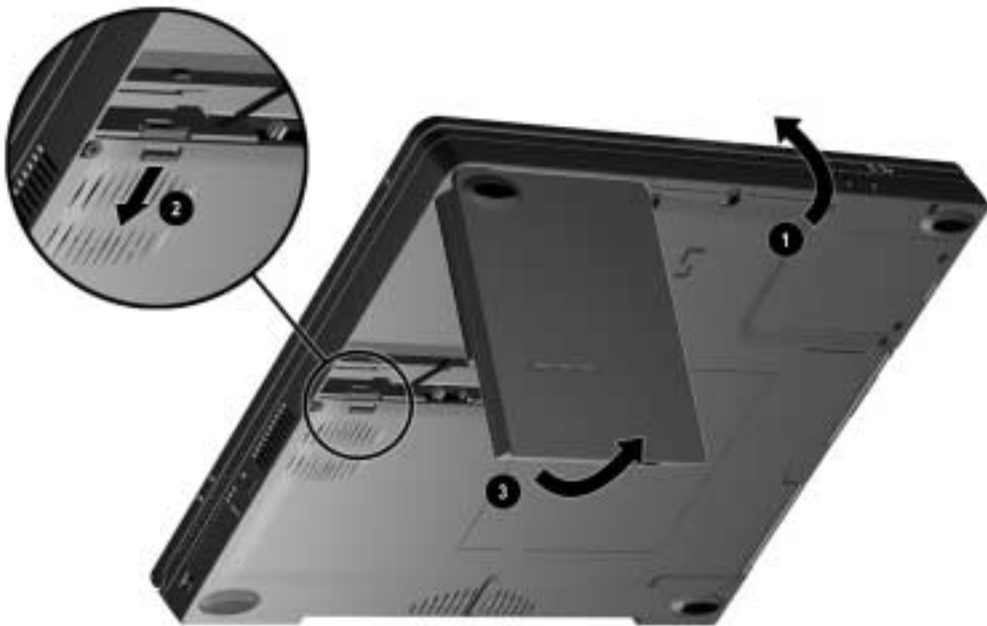
Figure 5-5. Removing a Battery Pack
