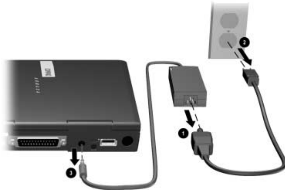
Figure 5-3. Disconnecting the Computer
