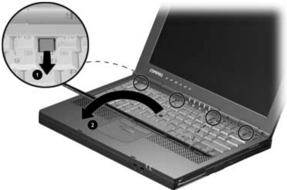
Figure 5-18. Removing the Keyboard
